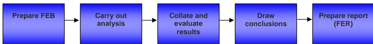
Figure 7.2 – Figure 1.1.2 of IFEG Typical fire engineering process
